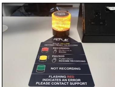
**Flashing amber:** If a scheduled, ad hoc or live stream recording is paused, the light will flash amber.
