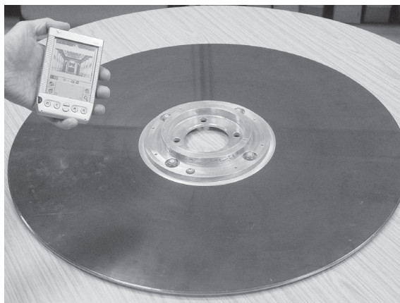
This steel disk platter from the original EMAS service held some 750kilobytes of information. The final EMAS service served up to 80 simultaneous users on a 15MIP machine with 64 megabytes of main memory—little more than that in the Personal Digital Assistant shown alongside the disk in the photograph.
